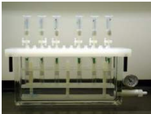
Figure 8.6: Typical Solid Phase Extraction Setup
